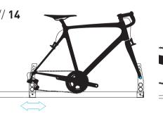
Adjust position of rear hub according to your wheel base. Place rear drop-outs on rear hub with correct upper axle adapter. Thighten your rear axel. Always choose lowest possible level at rear hub according to chain wheel size.
